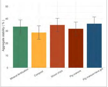
Figure 3. Stability of soil aggregates after incorporation of organic soil amendments; no significant differences measurable
