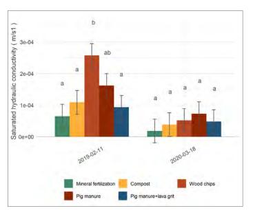
Figure 2. Water infiltration rate after incorporation of organic soil amendments; significant positive effect of wood chips
