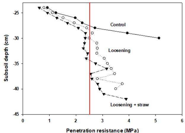
Figure 2. Changes in the penetration resistance upon subsoil loosening and loosening + straw incorporation. The red line (2.5 MPa) indicates the critical limit for root penetration.
